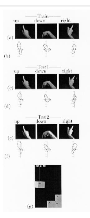
Subset of vocabulary of gestures used to control computer graphic crane. (a) shows the training set of gestures for the commands up, down and right. (c) shows a test set of the same gestures, under the same lighting conditions. (e) is a test set, made under different lighting conditions. (b), (d), and (f) are the corresponding orientation histograms. Note that the shapes look approximately the same as for the same hand
