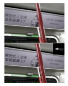
Figure 5: Top: A scene with a small blue. The patch selected by the user is indicated by the gray rectangle. Bottow: Output of our algorithm and the inferred blue kernel. Note the orisp text.
