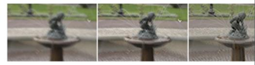
Figure 1: Left: An image spoiled by camera shake. Middle: result from Photoshop "unsharp mask". Right: result from our a
